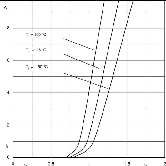
Fig. 1, Forward characteristics (typical values)
