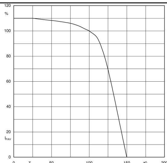
Fig. 2, Rated forward current vs. amb. temperature <sup>4)</sup>
