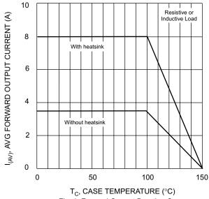
Fig. 1 Forward Current Derating Curve
